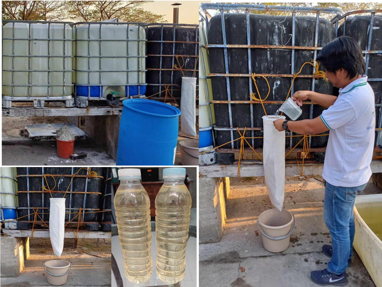
Trial on collection and filtration of magnesium/potassium chloride (Nigari liquid)
