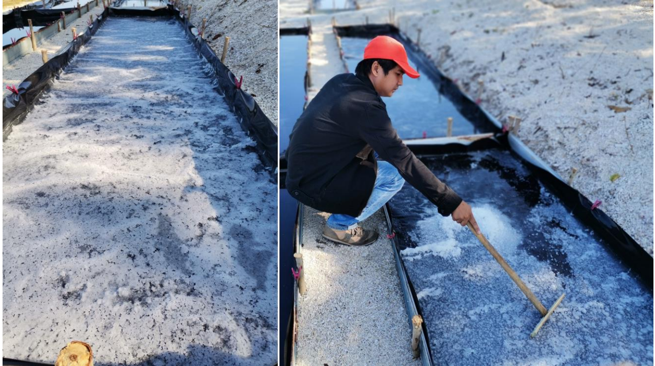
Harvesting of sea salt produced in HDPE platform
